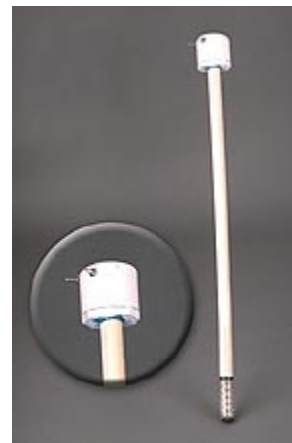
Fig. 8. Soil moisture sensors can be glued to the end of PVC pipe. Wire leads from the sensor are connected to bolts protruding from a PVC cap for easy access while taking readings. This installation allows the sensors to be retrieved and reused.
